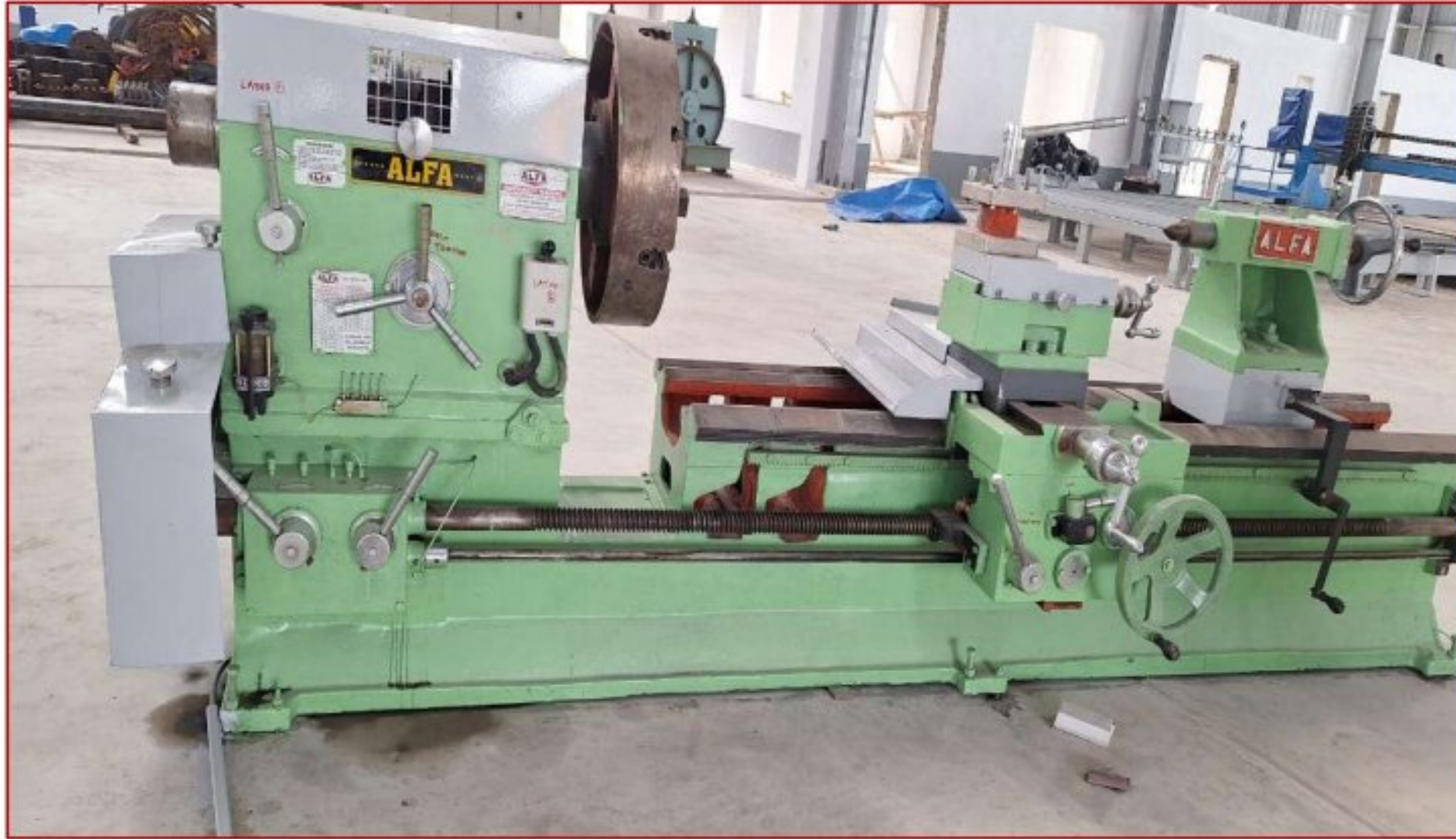
LATHE NO 1 LENGTH 12' & WIDTH 20"
