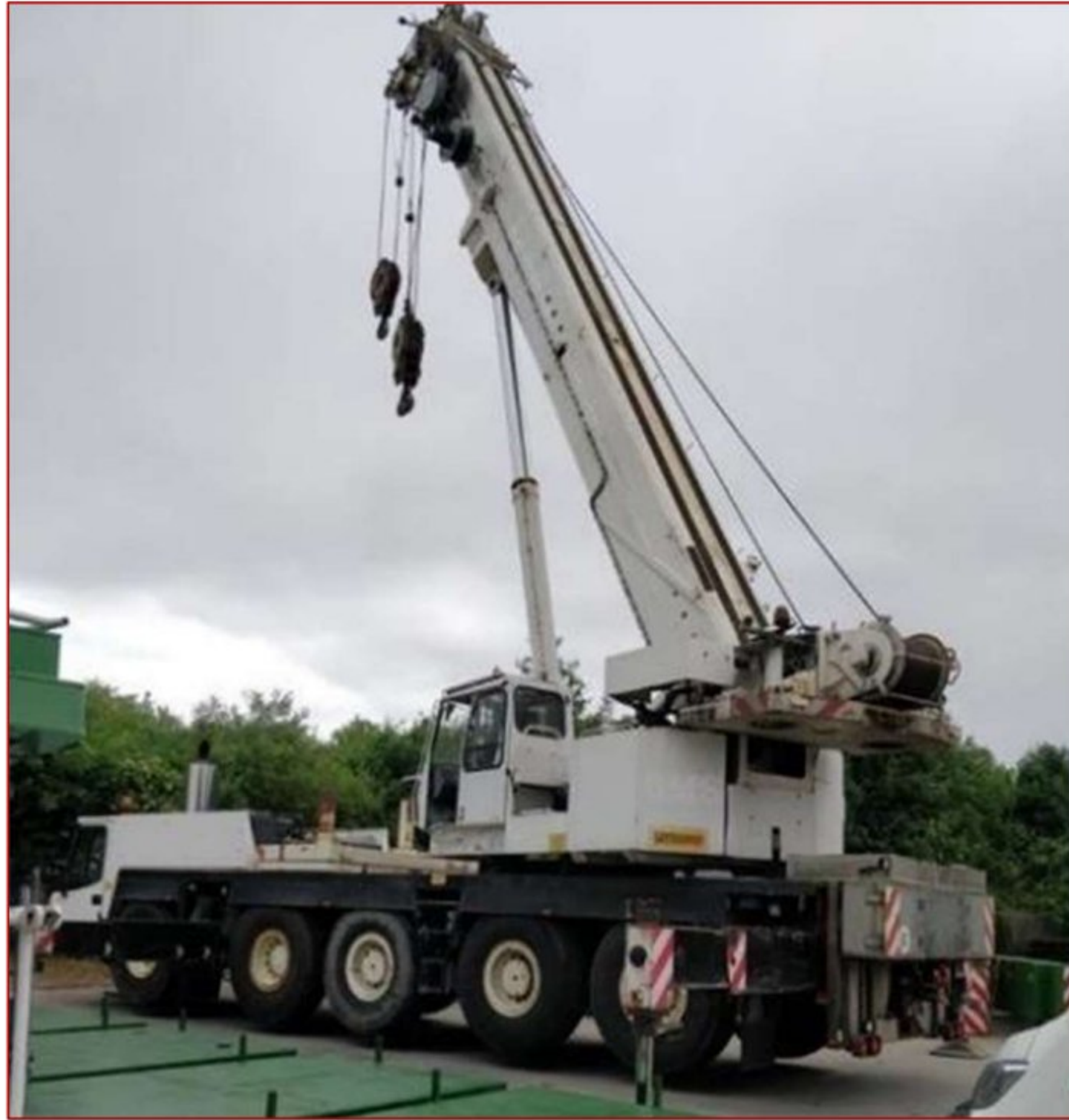
100T MOBILE CRANE Make: Grove, Model: GMK-5100, Capacity: 100 Ton, 50m Boom Height
