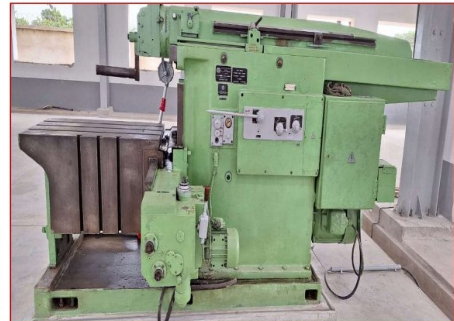
SHAPING MACHINE STROKE 10 MM (Min) & 1000 MM (Max)
