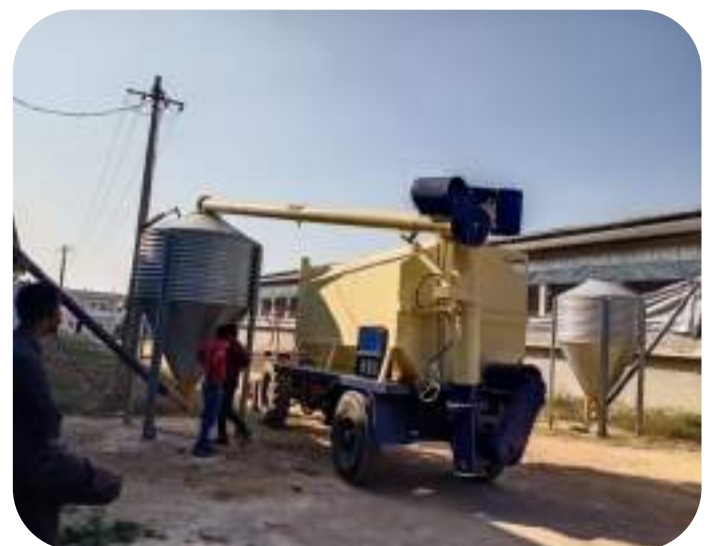
TRACTOR TANKER 5-6 TONS CAPACITY USED FOR CONVEYING FEED
