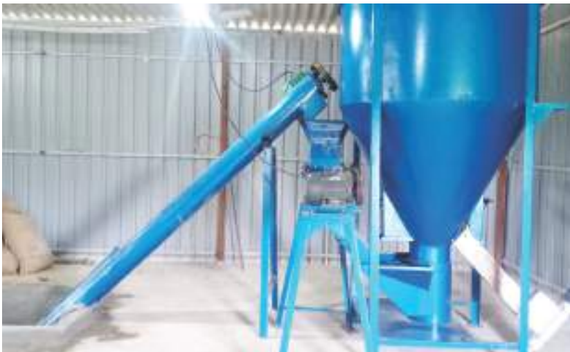
Vertical mixers are suitable for 5,000 to 50,000 birds. Designed for small farms.
