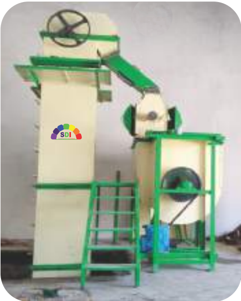
Horizontal Mixer (2-3 TPH) Power - 23hp, Area - 10ft* 10ft * 15ft Height
