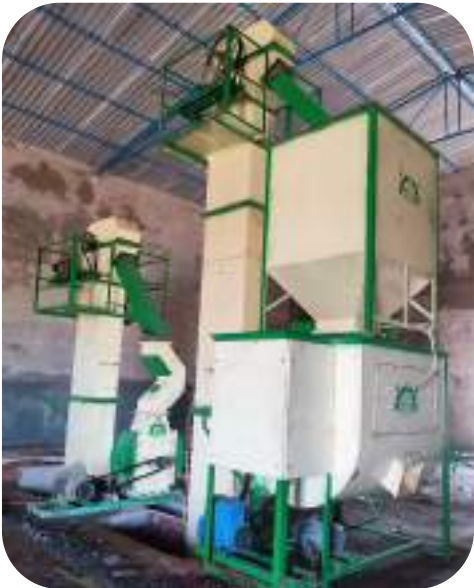
Full Plant With Horizontal Mixer 4-6 Tons Per hr, power - 36hp. Area - 8ft* 22ft Height
