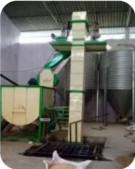
Mini Plant With Weighing Scale Power - 23hp, Area - 10ft* 10ft * 15ft Height
